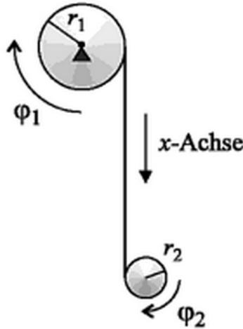
$$m_2 g = \left( \frac{m_1}{2} + m_2 \right) r_1 \ddot{\varphi}_1 + m_2 r_2 \ddot{\varphi}_2 \quad (\text{L.7})$$
