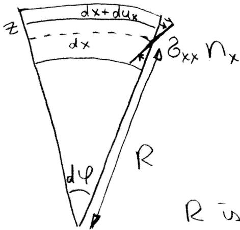
The length of the neutral surface  $dx = R d\varphi$  is unchanged.  $R$  is radius of curvature.
