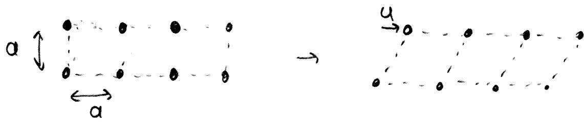
For small  $u$  the strain is  $\frac{u}{a}$  and stress is  $\mu \frac{u}{a}$ .
