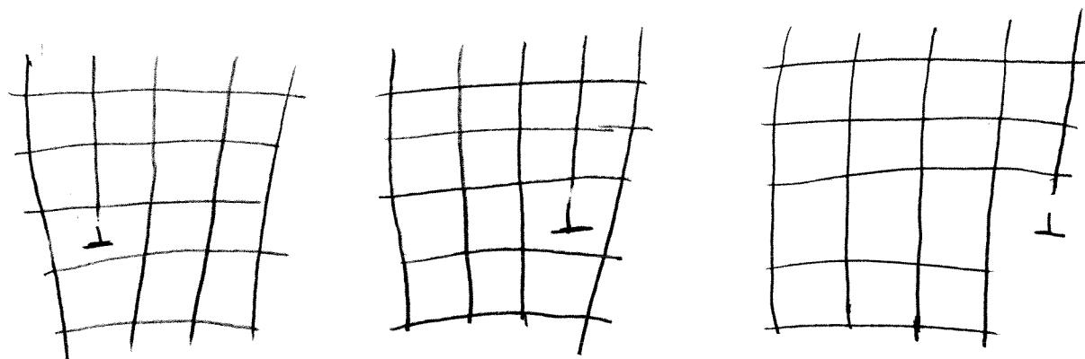
If dislocation moves through the crystal it produces shift of the upper half crystal by the unit vector  $\vec{b}$ . The shear that leads to the dislocation motion is much smaller than  $\mu$ . That is why  $\beta_m \ll \mu$
