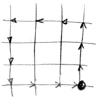
The same sequence of steps around dislocation will lead to displacement  $b$
