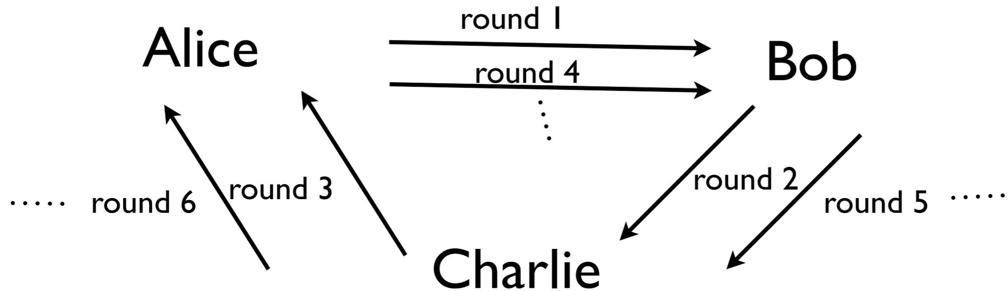
$$\Lambda(\rho) = \sum_{i_1, \dots, i_n} A_{i_1 \dots i_{n-2}} \cdots A_{i_1} \otimes B_{i_1 \dots i_{n-1}} \cdots B_{i_1 i_2} \otimes C_{i_1 \dots i_n} \cdots C_{i_1 i_2 i_3} \rho(\dots)^\dagger \otimes |i_1 \dots i_n\rangle \langle i_1 \dots i_n|$$
