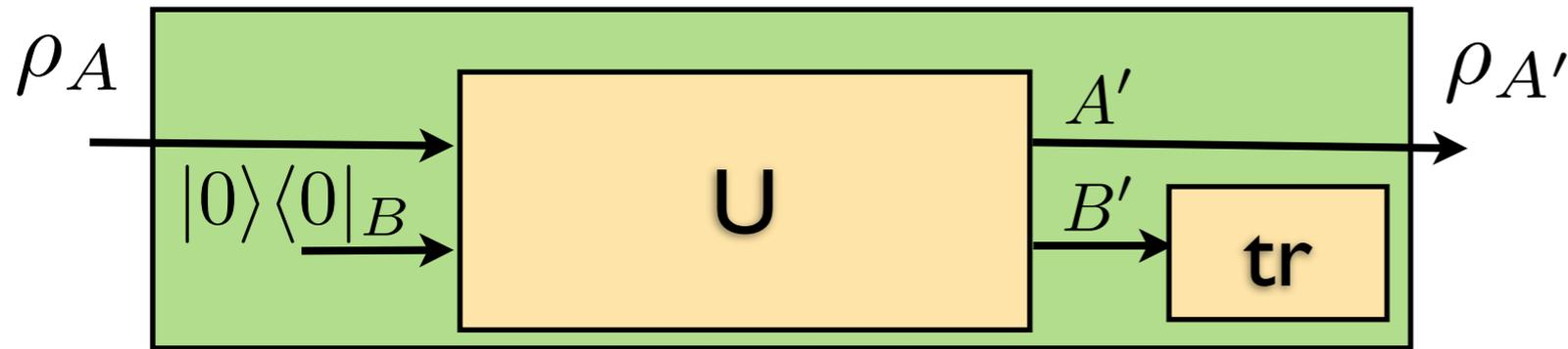
$$\Lambda(\rho_A) = \text{tr}_{B'} U(\rho_A \otimes |0\rangle\langle 0|_B) U^\dagger = \sum_i \langle i|_{B'} U |0\rangle_B \rho_A \langle 0|_B U^\dagger |i\rangle_{B'}$$
