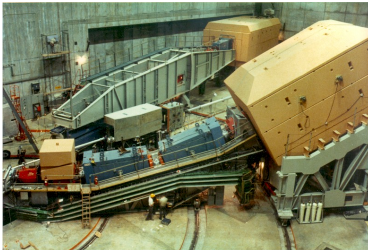
FIG. 2. (a) Plan view of End Station A and the two principal magnetic spectrometers employed for analysis of scattered electrons. (b) Configuration of the 8 GeV spectrometer, employed at scattering angles greater than 12^\circ .
