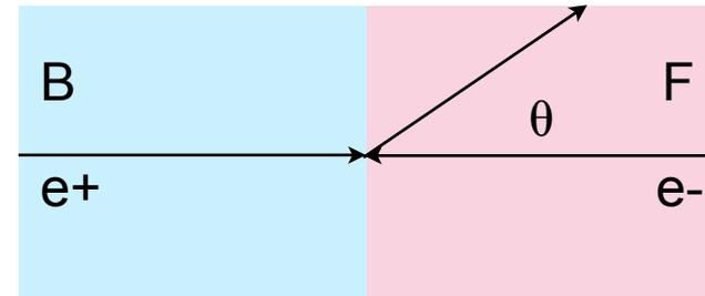
$$A_{\text{FB}} = \frac{3}{4} F_2/F_1 = 3 v_e a_e v_f a_f / (v_e^2 + a_e^2) \cdot (v_f^2 + a_f^2).$$
