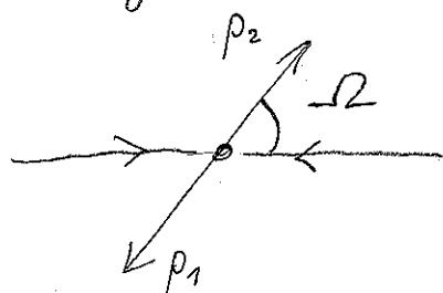
$$\frac{dG}{d\Omega} = \frac{1}{2 \cdot 2E_A E_B |v_A - v_B|} \frac{|\vec{p}_1|}{(2\pi)^2 4E_{CM}} |M|^2 \quad (32)$$
