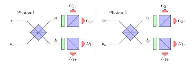
Here, blue squares represent polarising beam splitters (PBS) that transmit photons in  $|V\rangle$  and reflect photons in  $|H\rangle$  polarisation. Green rectangles represent half-wave plates (HWP) oriented at  $\pi/8$  angle, such that  $|H\rangle \to \frac{1}{\sqrt{2}} [|H\rangle + |V\rangle]$  and  $|V\rangle \to \frac{1}{\sqrt{2}} [|H\rangle - |V\rangle]$ . Red half circles represent single-photon counters.
